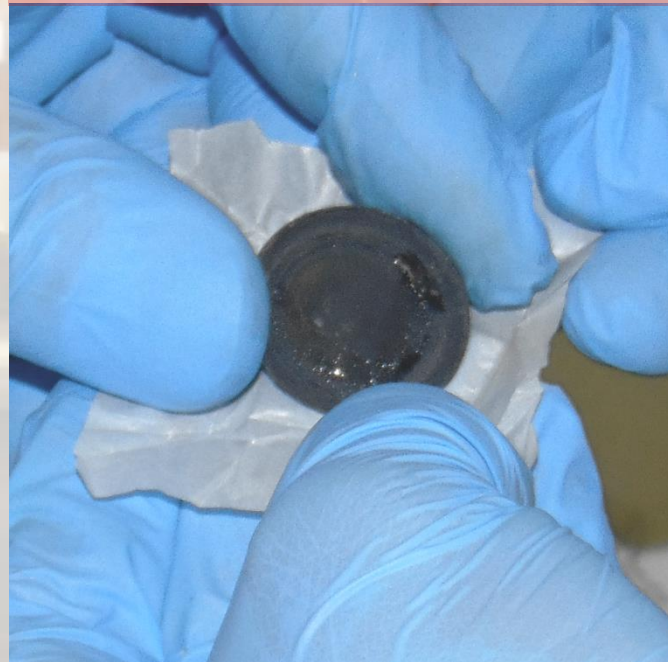
Detail of a sample of material extracted from Real Life Tester, visibly deteriorated after a test cycle.
